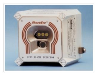
SharpEye CCTV Flame Detector is extremely sensitive. It can detect a  $1\text{ft.}^2$  (0.1m<sup>2</sup>) gasoline pan fire at 100 ft. (30m) in less than 10 seconds. The sensitivity is user-programmable, offering 4 ranges of detection.
