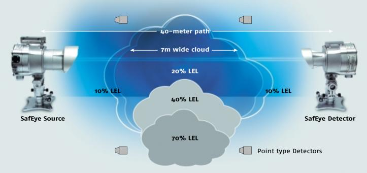
This scenario shows how matrix of Point' type detectors can miss a leak or eventually only see diluted gas levels whereas SafEye~700~Open-Path~will, in this case, measure 20%~LEL~x~7~m=1.4~LEL.m - well above 1~LEL.m alarm level
